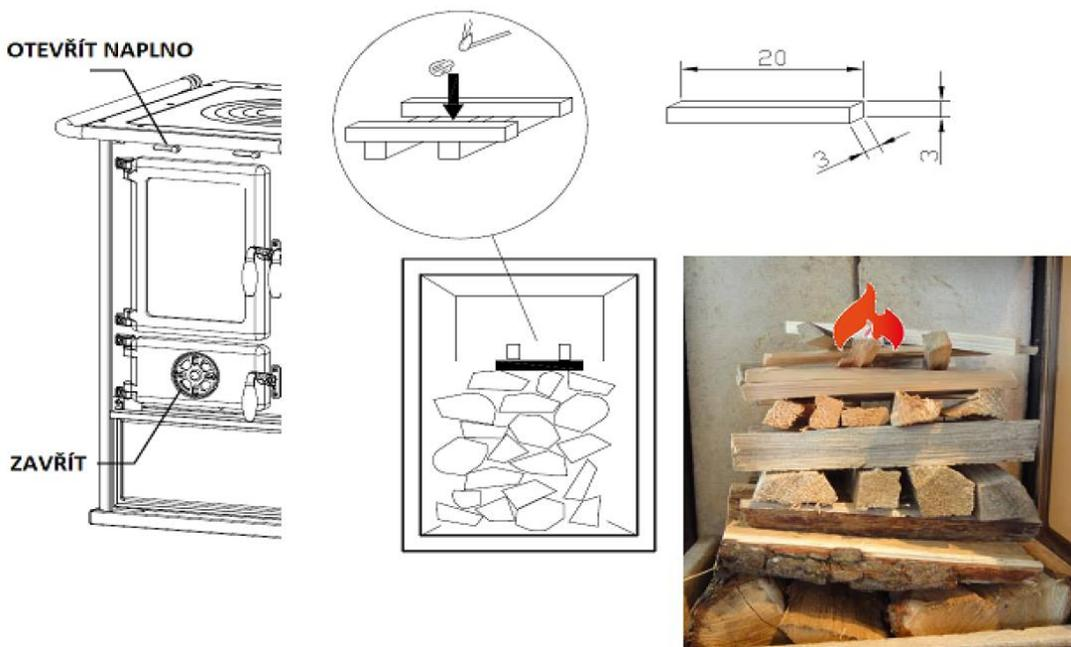
**NAUČTE SE ROZTÁPĚT V KAMNECH TZV. OD SHORA. DOCÍLÍTE TÍM RYCHLE ZAHŘÁTÍ SPALINOVÝCH CEST A KOMÍNU A SKLO BUDE KŘÍŠTÁLOVĚ ČISTÉ. PRIMÁRNÍ VZDUCH MĚJTE ZAVŘENÝ A SEKUNDÁRNÍ OTEVŘETE NAPLNO.**
