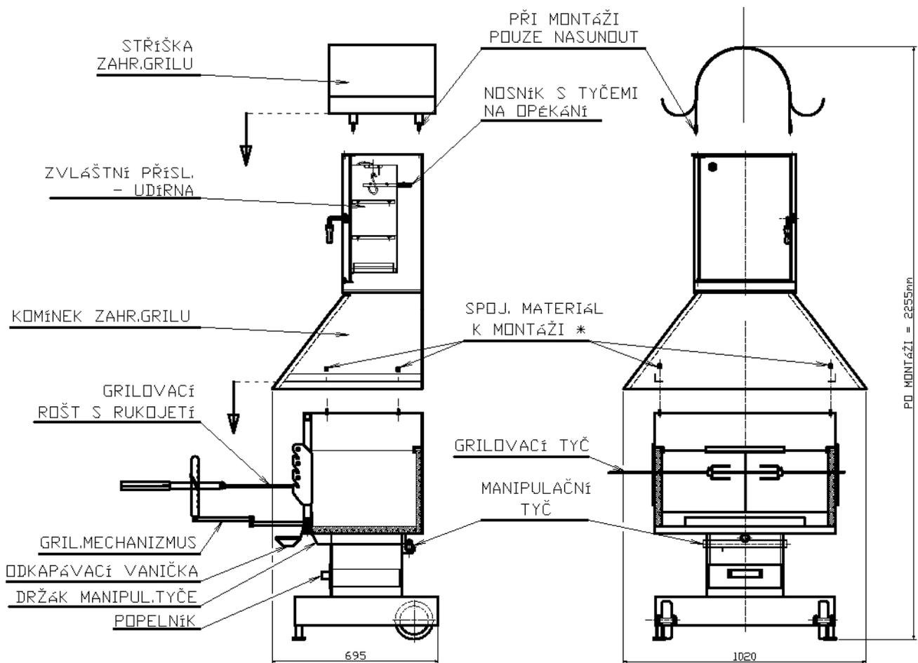
\* SPOJOVACÍ MATERIÁL = 4xPODLOŽKA  $\varnothing 6,4$  + 4x MATICE M6
