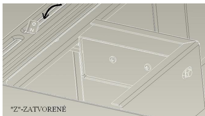
FIKO 70 Nostalgia B, Fiko 70 Ratio, FIKO 70 Plus Firing flap valve is closed
